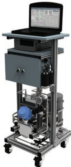
An automatic fuel flow calibration cart.
