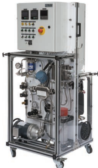
The RS438-200 diesel fuel flow measurement system.
